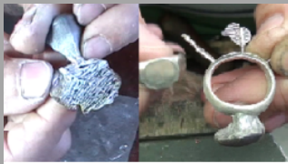
CUTTLEFISH CASTING (TWO TECHNIQUES)
