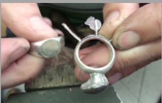
— CUTTLEFISH CASTING A RING
