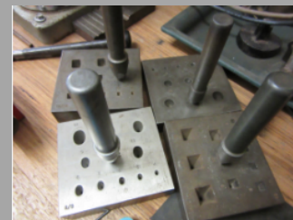
MAKING SETTINGS WITH COLLET BLOCKS
