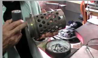
INVESTING FOR LOST WAX CASTING
