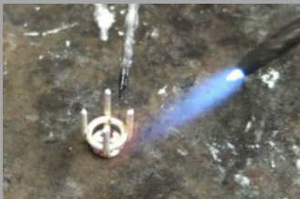
DOUBLE BEZEL FOUR CLAW SETTING
