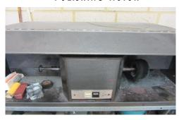
You can spend a fortune on a motor & extractor combination. But you can get by with an off the shelf 2800 RPM I/5 HP motor (a slight variation is fine) Just make sure it has tapered spindles or you can at least fix one on. Also be aware that a lot of dust is generated, so mask up. My compound of choice is Hyfin for cutting and Rouge for finishing. A grinding machine is also useful for shaping tools but do not combine polisher with grinder as your mops will get contaminated.
