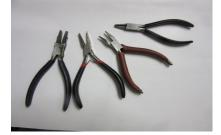
Round, Half Round, Chain nose and Parallel pliers are essential. But add a pair of Soft jaw (nylon) pliers for minimising tool damage as soon as you can.
