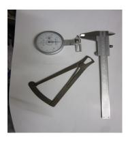
My choice of measuring devise is the gemstone dial gauge, it's quick and easy to read. Traditionally jewellers would generally use a steel Vernier or caliper gauge. Consider the digital or dial type.
