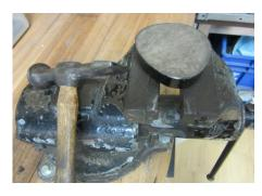
A good quality solid bench vice and a flat stake for forging will help to cold work metal. Find a good quality cross peen hammer. A large anvil is even better. I also use a nylon mallet for dent less forming rather than a rawhide mallet.
