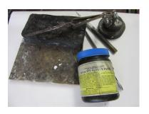
As well as a charcoal block I really like the ceramic soldering boards, they are clean and handle high temperatures well. You will also need soldering tweezers a third hand for setting up operation. I use the versatile Tenacity 4A flux paste. I pickle my work in warm sodium bisulfate & neutralize the acid with sodium bicarbonate.
