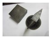
A steel bench anvil is really useful as you can form around the shapes. A steel block is good for heavy duty work
