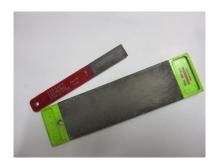
Eze-lap diamond hone & stone sharpeners are my weapon of choice, they are great for quick sharpen ups of drills and gravers. But if you are use to natural sharpening stones its fine to stay with it.
