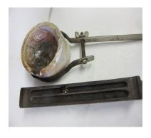
Once you have a crucible and ingot mold you can salvage your scrap metal and reduce the need to keep buying stock gauge precious metals. This set up is only applicable if you have an oxy/gas set up.
