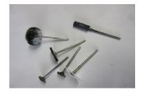
There are so many finishing discs & mops to choose from. I recommend a Split mandrel, a snap on mandrel (& Moors discs) Silicone carbide rubber polishers, Goats hair brush mops & cotton mops. This can be expanded on later.
