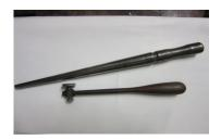
A good quality steel mandrel and a chasing hammer for shaping and sizing ring shanks is a must. You can also add a bangle mandrel to the list but it's not going to be necessary for Silver Level and fine jewellery making.
