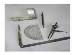
Good quality dividers are a must. A small steel rule, scribe set square and protractor for working out angles will be needed. Also add a scalpel to the list as this is a handy tool for marking out settings.
